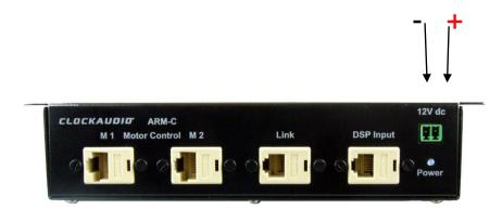
8. Turn on the DC supply to the controller box. The coloured power indicator will illuminate confirming that a supply is present. The motorised microphone may initially very slowly fully extend and then retract. This is normal as it will be auto-calibrating.
