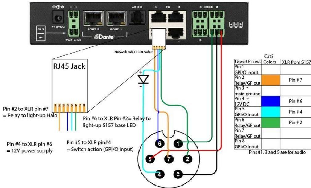
The diagram above shows the Halo microphone base, the S157, it connects the same way as the S135 but using Pin #4 for a 12 Volt supply to the Halo LED and output Pin #2 to turn it on.
