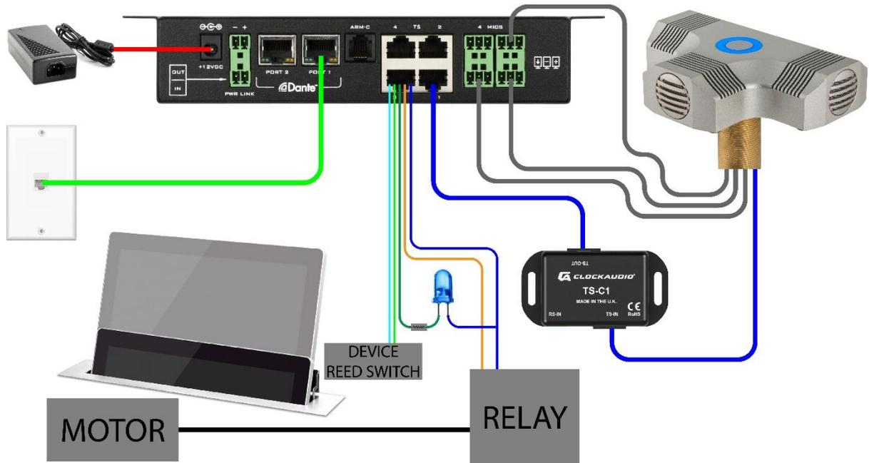
Pictured above, the CDT100 MkII is using output Pin #2 and the 12V supply from Pin #4 to trigger the Motor relay. The limit switch is sending a feedback via an input Pin #5 by grounding to Pin #3 and the LED is powered by Pin #4 and turned on by the internal grounding of Pin #6.
