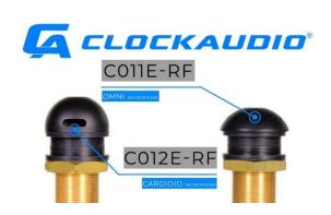
Both microphones are powered by a 9 to 48 volts phantom power adaptor which also includes filters that will eliminate all GSM frequencies from 800-1200 MHz. Frequency response 50 Hz to 18 KHz; Sensitivity -37dB +/- 3dB @ 1Khz (0dB=1V/Pa) Impedance 200 Ohms.
