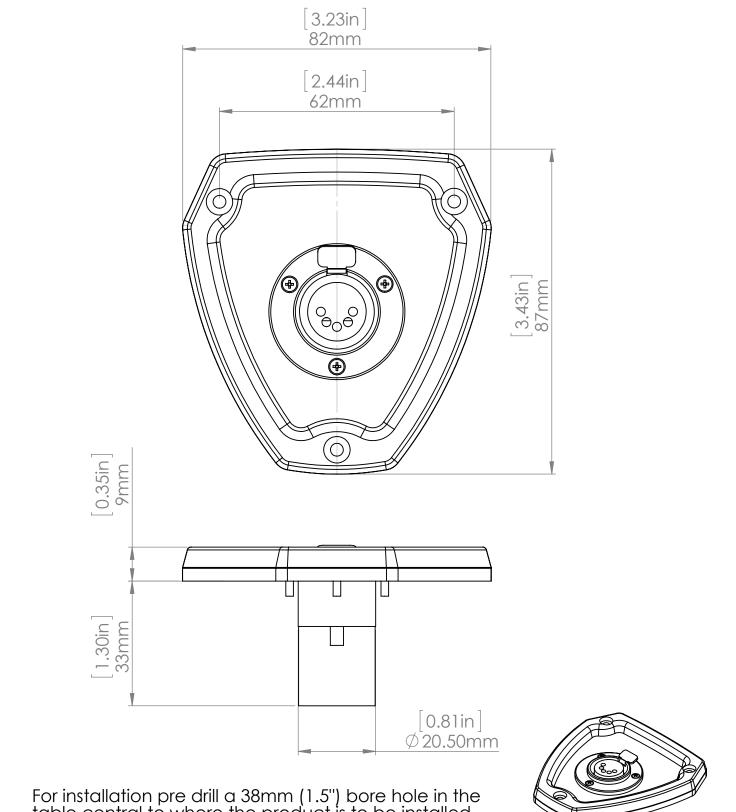
For installation pre drill a 38mm (1.5") bore hole in the table central to where the product is to be installed.
