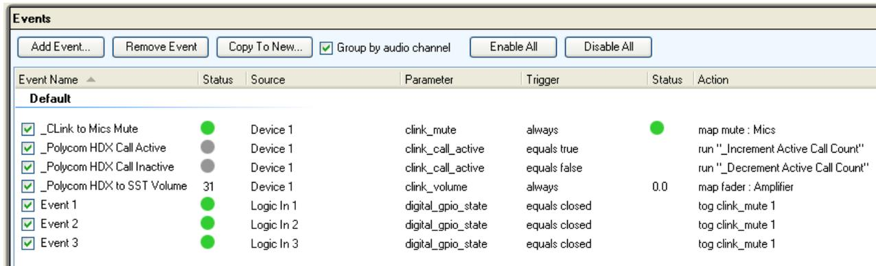
Figure 13. The resulting events page after the three logic input pins have been defined.
