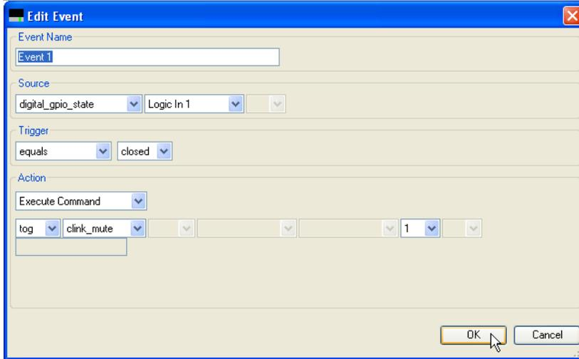
Figure 12. Adding and event for the first logic input pin.
