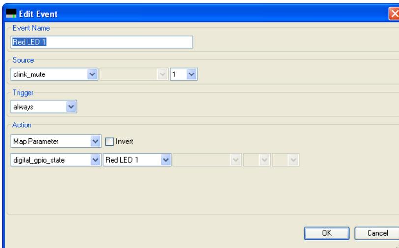
Figure 15. Event used to create the first Red LED output.
