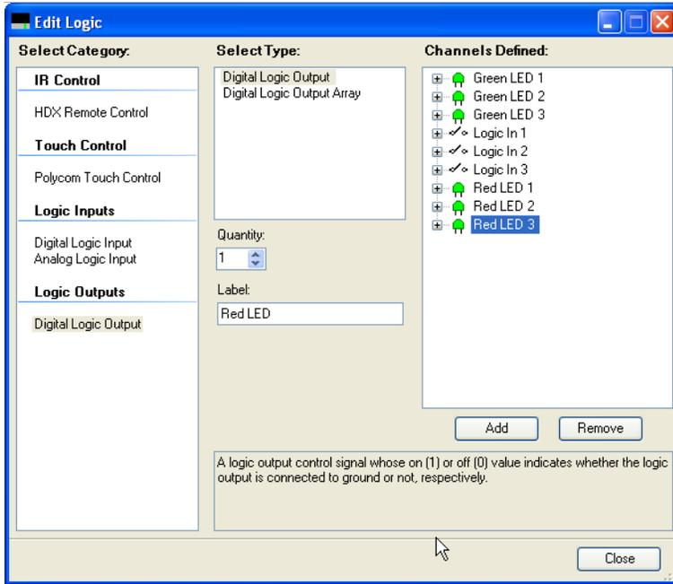
Figure 10. The resulting logic inputs and outputs.
