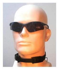
Special attention has been given to ensure a comfortable wear over long durations. The adjustable strap provides a good fit for various neck sizes. The transducer housing connector band is also adjustable to set the desired interhousing spacing. Additionally, it is ergonomically designed to avoid the thyroid notch, otherwise known as the "Adam's Apple". Cable is steel reinforced to provide high strength with minimum size & weight.
