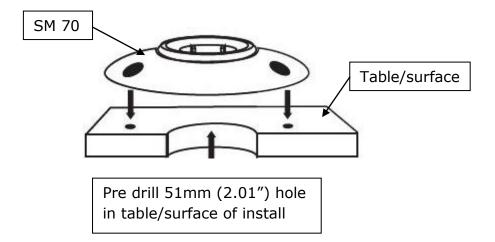
Installation of SM 70 through table shock mount
