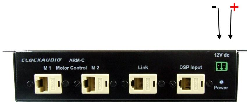
8. Turn on the DC supply to the controller box. The coloured power indicator will illuminate confirming that a supply is present. The motorised microphone may initially very slowly fully extend and then retract. This is normal as it will be auto-calibrating.
