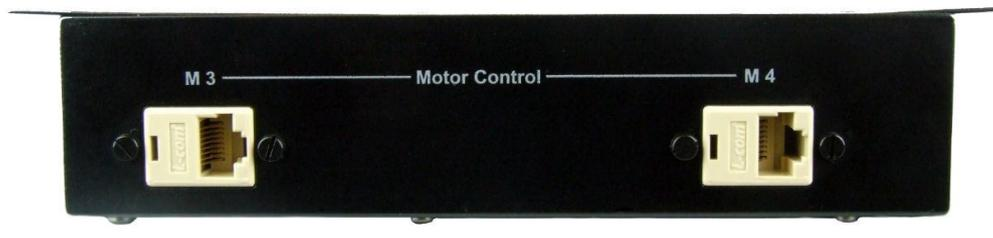
If the RJ12 cables need to be lengthened readymade / off the shelf extension cables are freely available at your high street electrical retail outlet. If cables are to be handmade then connections are made to pins 2 (Live) & 1 (Ground) shown below all other pins are not used.
